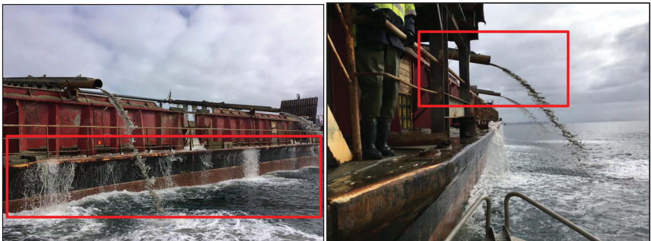
Figure 5.1: Hopper Weir Board (left) and Overflow Sample (right) Locations, indicated by Blue Rectangle
