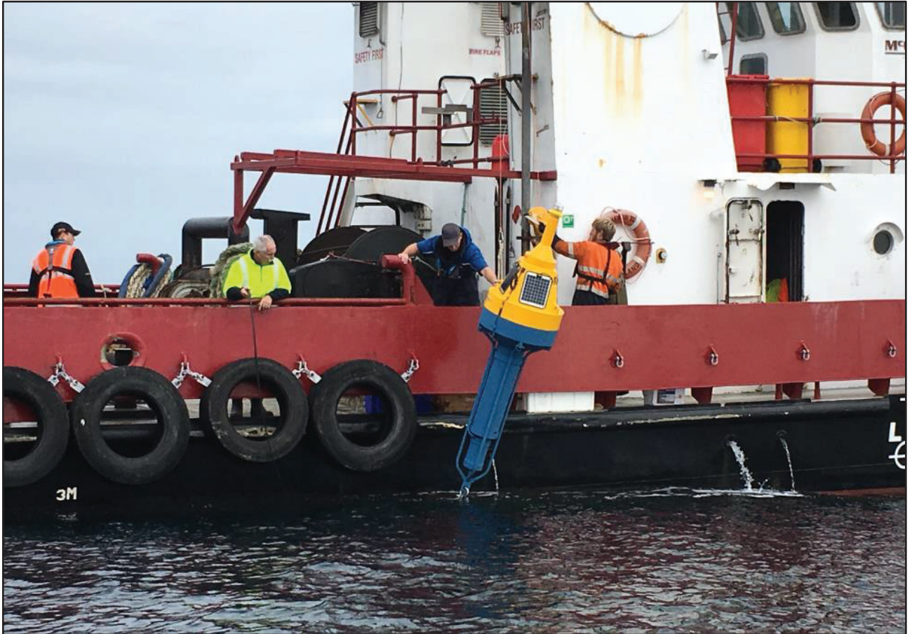
Figure 4.3: Deployment of ADCP and WETlabs WQM Devices
