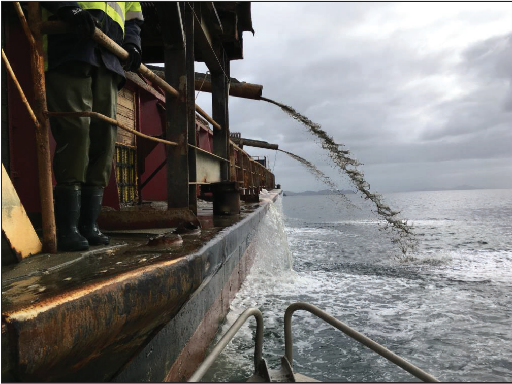
Figure 3.1: Discharge from the Dredge Vessel of Spoil from Overhead Flumes and from the Deck Over-Hopper Weir Boards
